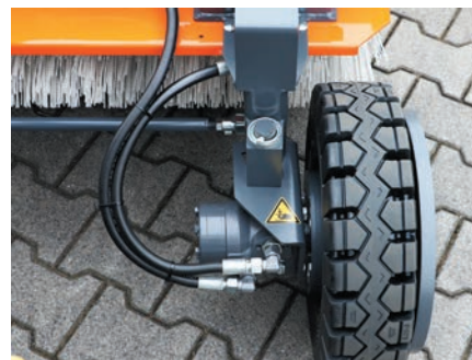
Efficient steerable wheel drive (hydraulic)
