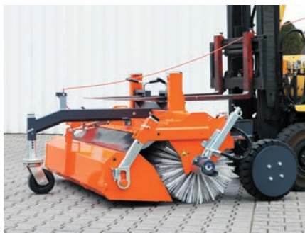
Collection container - emptying via rope
