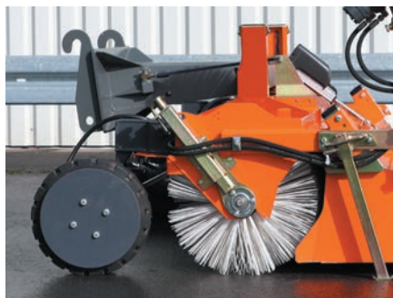
Stepless spindle adjustment of the main brush
