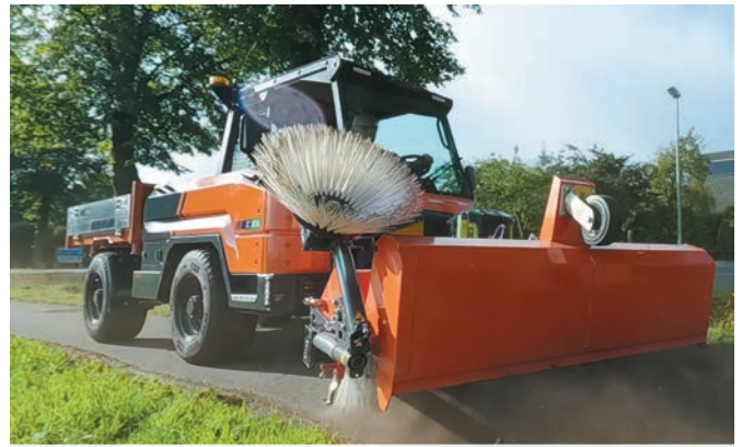
Sweezy® 580 Dual E with collection container in the proven Dual system, in this case free sweeping with an open collection container
